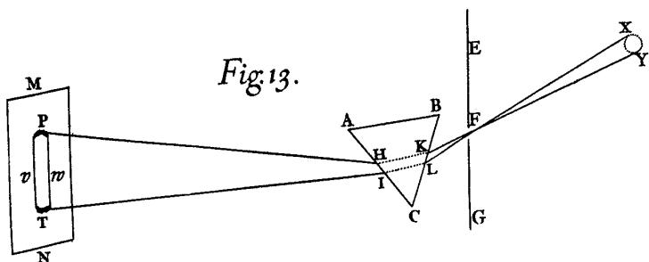
Fig. 1: Newton's basic experiment demonstrating the elongated spectrum. The image is taken from Newton's Opticks, Book 1, Part 1, Proposition 2, Experiment 3 (1704/1979:27).
