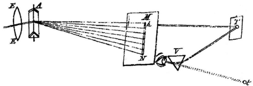
Fig. 4: Experiment 12 from Opticks, Book 1, Part 1, Proposition 5 (Newton 1704/1979:73). In Part 2, Proposition 2, Newton states that this experiment proves color immutability (1704/1979:122). The graph is taken from Shapiro 1996:116. In his trials in 1714, Desaguliers uses this experiment to show color immutability.
