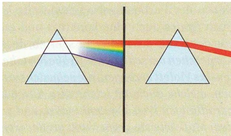
Fig. 5: Illustration in a contemporary German physics textbook for High School students. The image resembles the experimentum crucis and is supposed to illustrate that original colors cannot further be decomposed (Boysen et al 1999).
