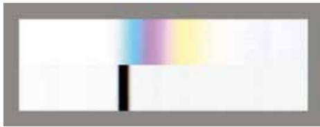
**Fig 17** Nussbaumer's black synthesis [I.N. 2009]. The top of the figure shows a picture of the complementary spectrum. The bottom shows a picture of it taken by a camera through the refracting prism. All the colours of the complementary spectrum converge and mix to black.
