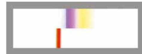
**Fig 19** Nussbaumer's red synthesis [I.N. 2009]. The top of the figure shows a picture of the complementary spectrum from which the left turquoise part is removed. The bottom shows a picture of this fragmented spectrum (without turquoise) taken by a camera through the refracting prism. Purple and yellow from the complementary spectrum (all its colours except turquoise) converge and are mixed to red.
