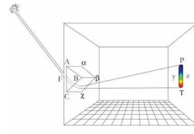
**Fig 1** Newton's white analysis (1672) [colour graphic by Ingo Nussbaumer based on a drawing in Newton's sketch book; Newton's original graphic is printed in Lohne [LN]: 126/7, "Figure 1"]. Rays of light are sent through a hole in the window shutter (F) into a prism. The light is refracted and split into its multi-coloured parts.
