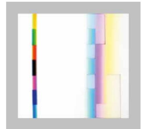
**Fig 22** *Nussbaumer's counterpoint to the original seven-fold colour synthesis* [I.N. 2009]. If you look through a prism at the screen with its windows of brightness (right half) when it is illuminated by the complementary colours, you see again all six main colours, only in a different order. Top: yellow, green, red – bottom: purple, blue, turquoise. The black synthesis is in the middle. If you switch the top and the bottom in this picture, you get the exact complement to Fig. 14.
