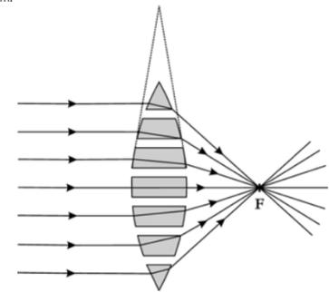
**Fig 5** Lens theoretically composed of prisms [the figure is from a high-school text book, Dorn et al [PM]:238/9 (Figure 239.2), redrawn with alterations by I.N. 2009]. The figure bears the cheerful caption "convex lens composed of prism pieces", and that although it looks like prism hide-and-see, not like a clear representation of a collection of prisms.
