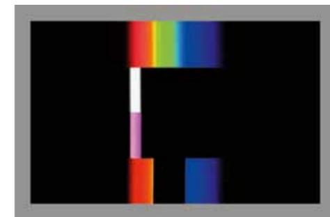
**Fig 11** Comparison of the simultaneous white and purple syntheses [I.N. 2009]. The results of looking through a prism at the starting image (Fig. 10) appear in the middle (rows 2 and 3). The photograph of these results proves that both syntheses are exactly the same size.
